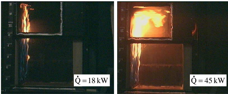
Fig. 3. Flame shapes in naturally ventilated atmosphere.
