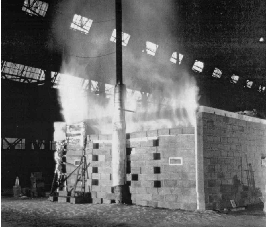
Figure 6.40 Natural Fire Tests in Large Compartment BRE, UK, 1994 - Test 6 V_f=1.2\text{m}^{5/2} - q_f=350\text{ MJ/m}^2
