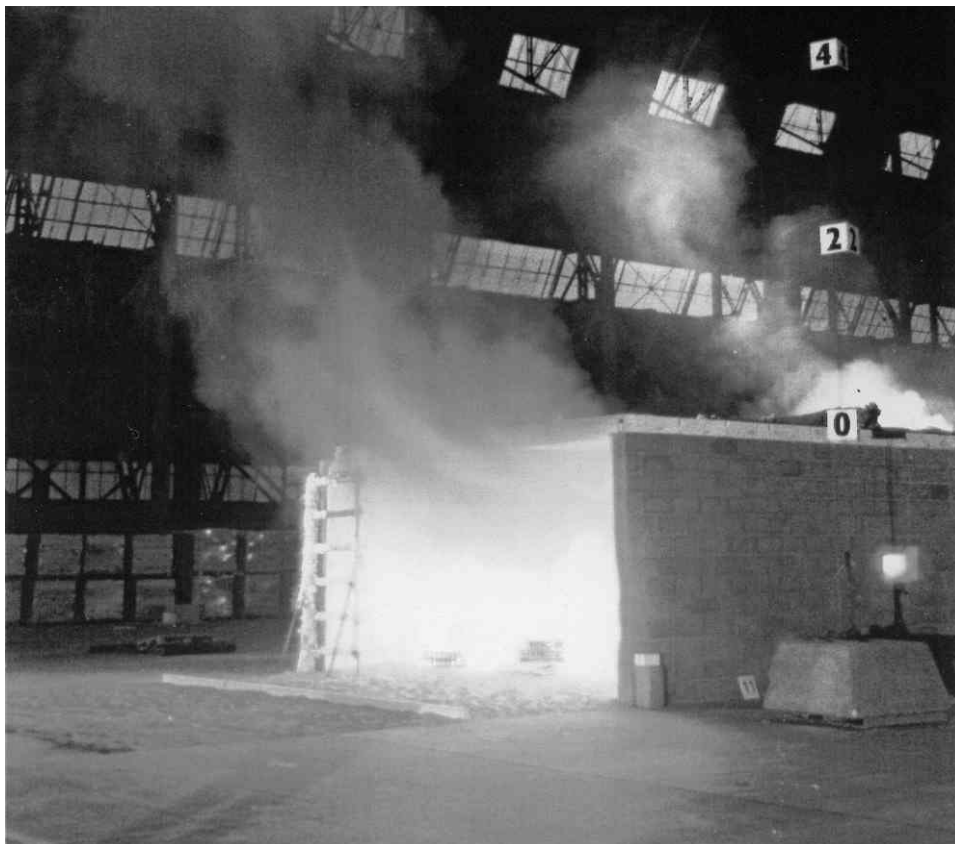
Figure 6.41 Natural Fire Tests in Large Compartment BRE, UK, 1994 - Test 2 V_f=25.5\text{m}^{5/2} - q_f=350\text{ MJ/m}^2
