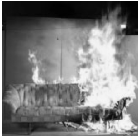
Figure 2.10 Sofa fire. The RHR at this point is about 800kW. (Sundström, 1997)
